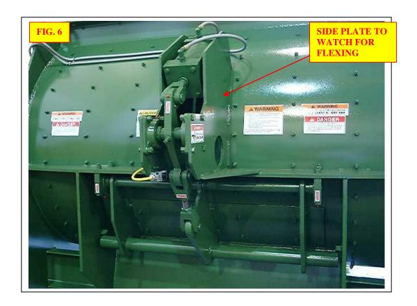
The side plates where the bearings for the locking lever are mounted will flex slightly when closing the door. If they flex too much the tension on locking lever arm needs to be adjusted. Shorten the rod assembly to relieve tension. Over time too much tension will crack the welds. (**See fig. 6**)
