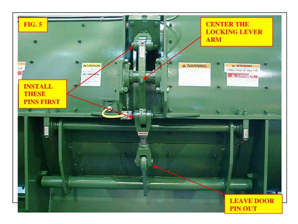
Install cylinder pivot pin, and the pin holding the clevis assembly to locking lever arm.
